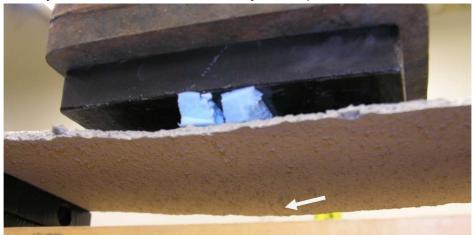
The beam was continued to be loaded until failure
