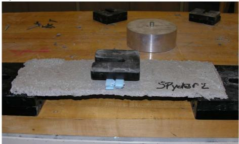
Loads was slowly incremented until the beam yielded (formation of first crack-below)
